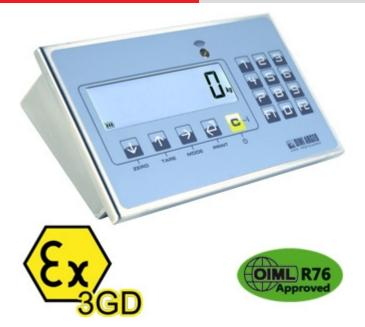
Easy to programme and use, versatile and high performing weight indicator, with IP68 stainless steel case. Ideal for using in areas classified as hazardous with protection methods according to II 3G Ex nR IIC T6 Gc X II 3D Ex tc IIIC T130°C Dc IP68 X. CE-M approvable (OIML R-76/EN 45501).
