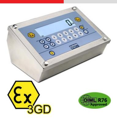
Weight indicator for areas classified as hazardous with protection methods according to: ATEX II 3G Ex nR IIC T6 Gc X ATEX II 3D Ex tc IIIC T130°C Dc IP68 X.
