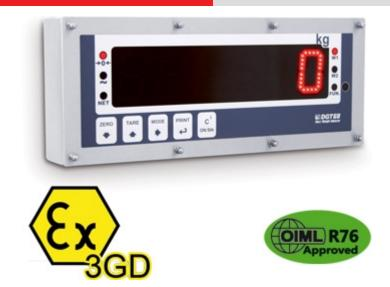
Weight indicator/ repeater particularly suitable for use in hazardous environments, where it's necessary to view the weight from a distance at any angle. Usable in areas: ATEX II 3G Ex nR IIC T6 Gc X ATEX II 3D Ex tc IIIC T130°C Dc IP68 X. Fitted with a very bright 60mm LED matrix display and IP68 stainless steel case. CE-M approvable (OIML R-76 / EN 45501).
